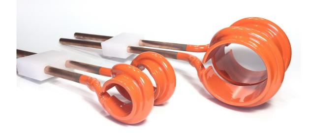
All solid state coils feature a coating of high temperature epoxy. This finish is very durable and can withstand very high temperatures. The coils are assembled with electrical grade copper parts and soldered with highly conductive silver solder.
